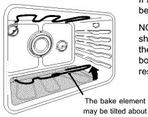
Fig. 2 4 or 5 inches to clean oven bottom
